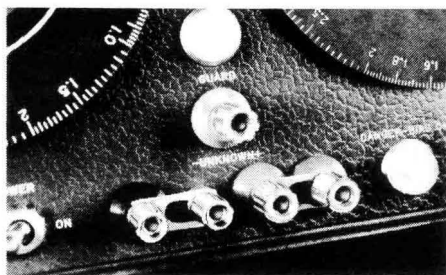
Figure 3-1. UNKNOWN and GUARD terminals on the bridge.
